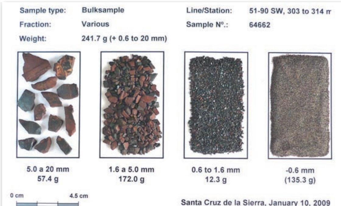
Foto 01: Concentrates of different fractions of bulk sample N°. 64662
