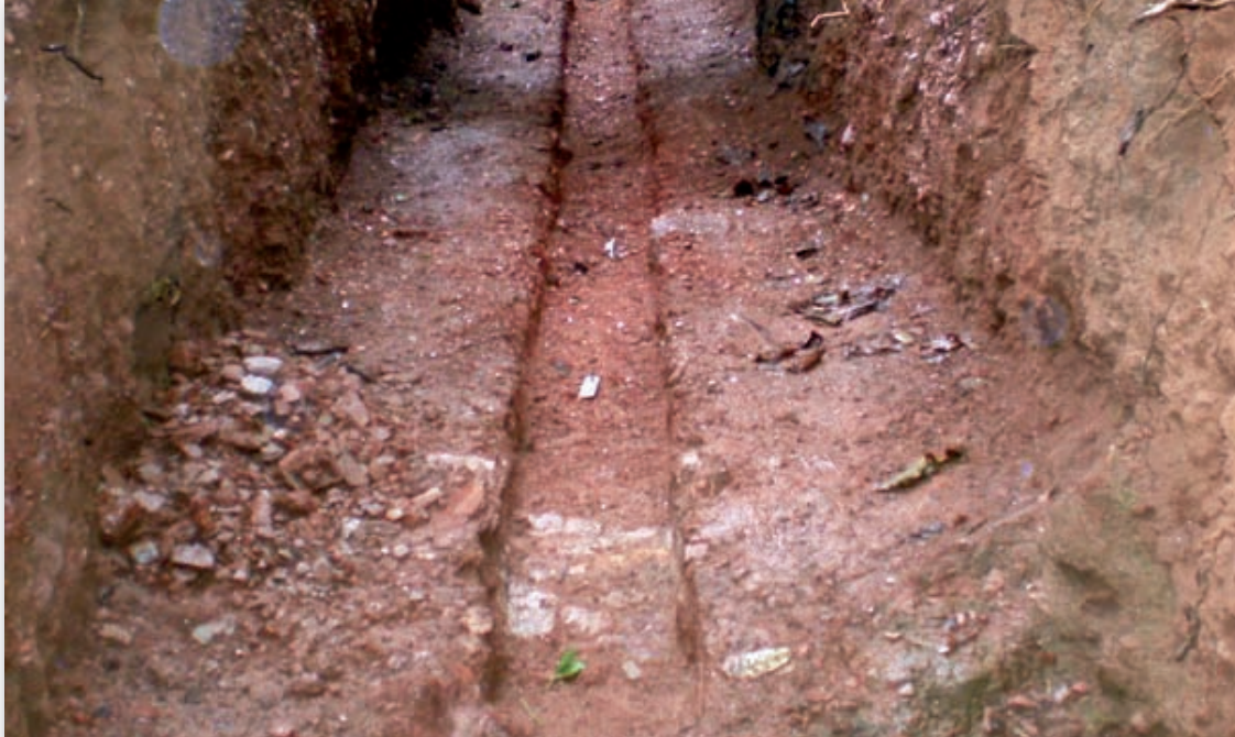
Photo 01: Horizontal sampling channel, width 0.15 m, depth 0.10 m, total length 15.0 m, line 52-00 SW
